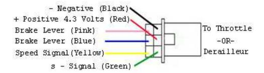
The Six Wire Connector is a combination of the Throttle Connector, Brake Lever Connector, and the Speedometer Connector. The Throttle wires (BLACK, RED, and GREEN) are required for the controller to function properly. The Brake Lever wires (PINK and BLUE) and the Speedometer Signal wire (YELLOW) are optional connections.
